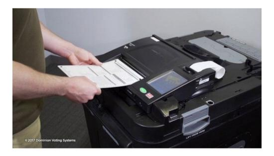
The Dominion ImageCast Precinct (hereinafter referred to as "ICP") stores ALL information on 2 compact flash cards, each of which is an identical copy of the other for redundancy. The ICP has no accessible internal hard drive or storage for election information besides the twin compact flash cards.
